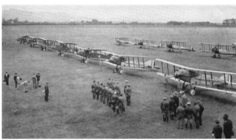
Aircraft of the New Zealand Permanent Air Force, Wigram, 1927. The types of aircraft are ( front row, left to right ) DH9, DH4, and Bristol Fighters; ( back row ) Avro 504K
