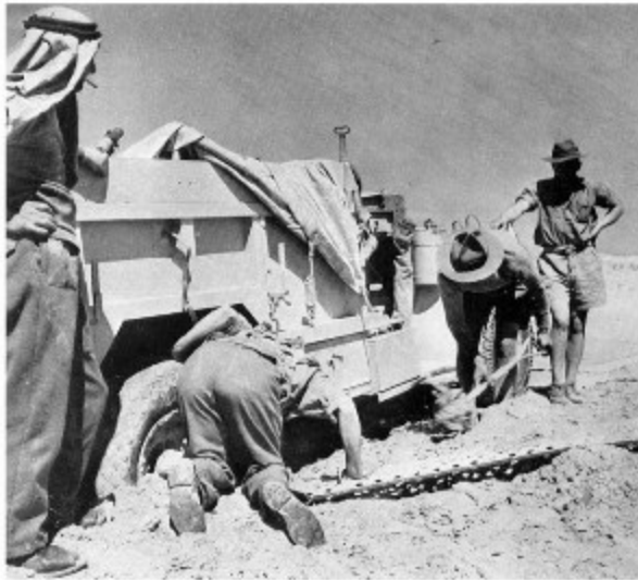
DIGGING OUT Perforated steel channels and canvas sand-mats were placed under the wheels and, with every man pushing, the truck was extricated two or three yards at a time.
