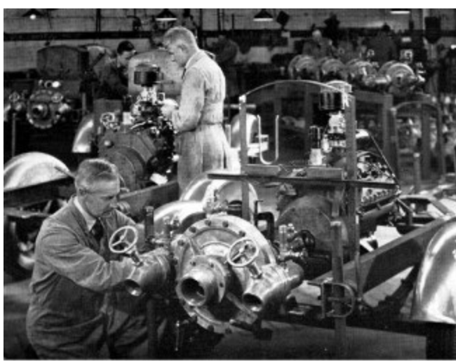
MANUFACTURE OF WAR EQUIPMENT Trailer fire pumps for the Far East forces
