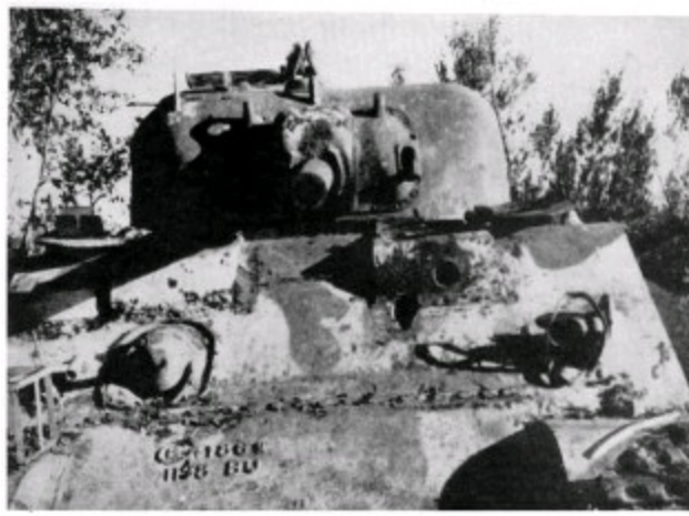
A knocked-out Sherman tank at Perano. Anti-tank shells have penetrated the driver's position. This was the regiment's first casualty in its first action in Italy (see pages 338-9)
